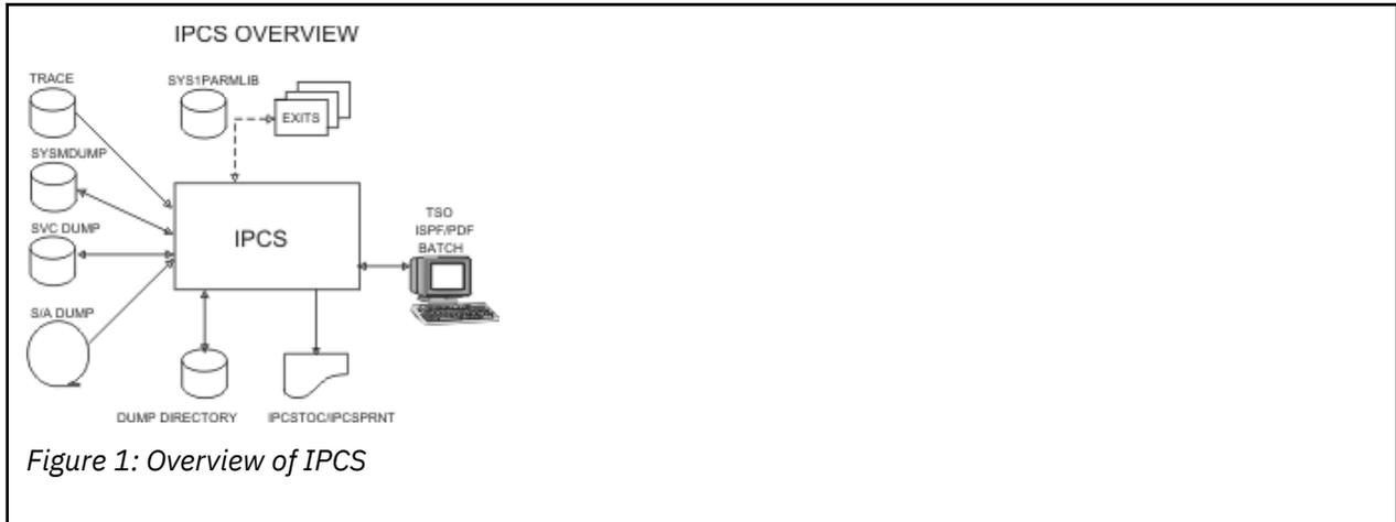
IPCS accepts unformatted dumps and traces as input. It uses members of parmlib to locate control block models and exit routines. The models and routines allow IPCS to format and analyze the contents of the dump or trace data set. IPCS produces three types of output: symptom strings placed in the headers of dump data sets, control block symbols and mappings of storage saved in a dump directory, and formatted reports that the user can view at a terminal or print.
